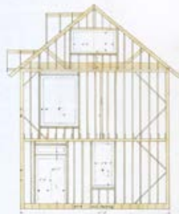
Framing East Elevation Scale 1/8" = 1'-0"
